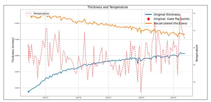
Figure 3: Misleading Thickness Increase Due to Active Corrosion
