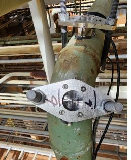
Figure 1: Ultrasonic Sensors with Mounting Fixtures on 2-inch Piping
