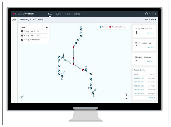
Figure 5: Circuit-Level Visualization of CML Status
