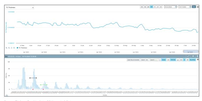
Figure 6: Thickness Trend Analysis of CML on 2-Inch Piping
