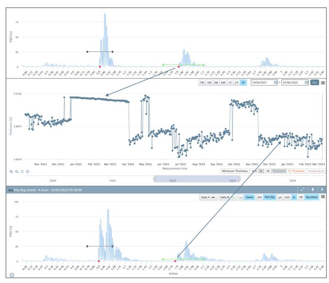
$Figure\ 2: Impact\ of\ Corroding\ Surfaces\ on\ Ultrasonic\ Waveforms\ and\ Thickness\ Measurements$
